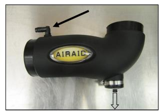
12. Install the Barbed Fitting (#21) into the Intake Tube as shown. Remove the aluminum Plug in the Tube if the Resonator is to be retained.
