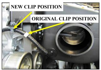
10. Route the MAF harness into the Airbox and reconnect the sensor inside. Seal off the access port with the Grommet from step 9. Relocate the plastic clip on the wire harness 1 1/4" back to take up any slack that might allow contact with the accessory belt.
