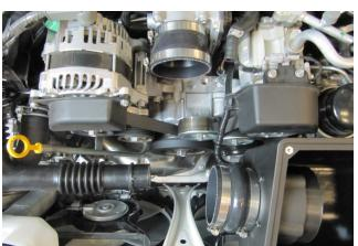
11. Place the Hump Hose (#5) and two #52 Clamps (#20) onto the Filter Adapter and the Reducer (#6) with one #52 and one #44 Clamp (#19) on the throttle body. Leave the clamps loose for now.
