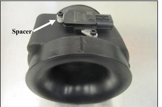
**4.** Transfer the Mass Air Flow sensor into the Filter Adapter (#4) and secure using the two 8-32 Socket Head Screws (#17) and Spacers (#18).
