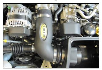
**13.** Install the Intake Tube and tighten all of the clamps. Connect the crank case breather to the Barbed Fitting and secure it using the OEM spring clamp. Insert the resonator into the Intake Tube and tighten the clamp.
