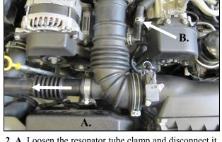
**2. A.** Loosen the resonator tube clamp and disconnect it from the intake. **B.** Compress the spring clamp on the crank case breather line and disconnect it. Remove the intake tube from the vehicle.
