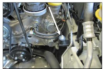
**6.** Install the CAB Mount (#16) into the airbox bracket on the inner fender. Hand tight is sufficient.
