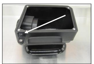
7. Mount the Airbox Bracket (#10) as shown, using one 1/4-20 Button Head Screw and a 1/4" Flat Washer. Transfer one factory airbox mounting grommet and steel sleeve from step 3 into the Airbox Bracket.
