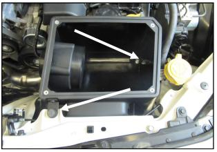
**8.** Slide the CAB Mount stud through the hole in the Airbox bottom and secure it using the M6 Flange Nut (#15) and a 1/4" Flat washer. Reuse one 6mm airbox bolt from step 3 to join the Airbox Bracket to the core support.
