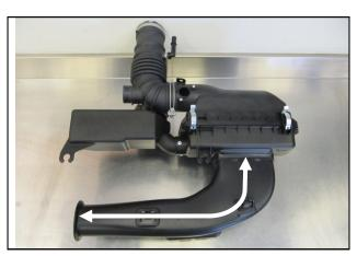
19. Install Option Two: OEM air inlet removal. While not necessary, maximum power is acnieved by removing the OEM inlet from the vehicle.
