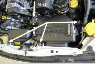
**3.** Disconnect the Mass Air Flow sensor, or MAF, in the airbox. Remove the three 6mm bolts securing the airbox assembly and remove it from the vehicle.
