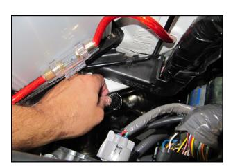
18. Place the Firewall Grommet into the bulkhead. . NOTE: The resonator Delete option has no positive or negative effect on performance
