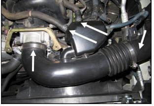
2. A.) Using a pair of pliers, compress the spring clamps on the PCV breathers and them slide back. Disconnect the breathers from the factory intake **B.)** Loosen the two clamps on the factory intake tube and remove it from the vehicle.
