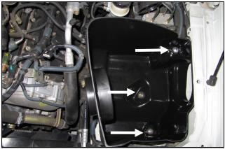
6. Set the CAB assembly inside the engine compartment,
