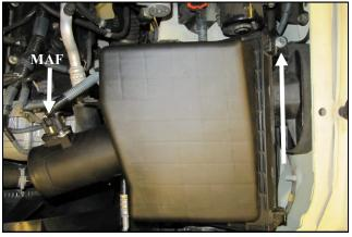
3. Disconnect the Mass Air Flow sensor, or MAF, and separate the wiring harness from the airbox lid. Using a 10mm socket, remove the single bolt securing the airbox. Lift straight up on the airbox assembly and unseat it from the mounting grommets on the inner fender. 4WD models will need the differential breather disconnected from the airbox lid.
