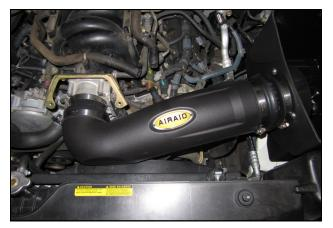
10. Install the Airaid Intake Tube into the Hump Hose first, and then into the Reducing Coupler. Adjust for fit, and tighten all four Hose Clamps.
