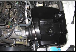
7. Install the threaded 5/8" Barbed Fitting (#15) into the Airaid Intake Tube (#2). Transfer the Mass Air Flow sensor from the factory airbox, into the Airaid Intake Tube and secure using the two 8-32 Button Head Screws. Do not attempt to reuse the factory screws.
