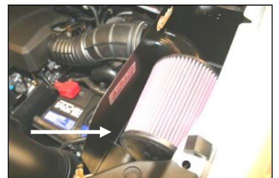
6. Install the Airaid Premium Filter (#1) onto the Quick Fit Panel Tube as shown, and tighten the clamp.
