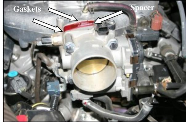
4. Install the spacer (#1) (with the flat side of the helix bore facing the throttlebody) between the intake manifold, and the throttlebody with one of the supplied gaskets (#2) on each side of the spacer. Insert four 8mm x 75mm Hex Bolts (#3), and 8mm Flat Washers (#4) through the throttlebody, Poweraid Spacer, and into the intake manifold. Using a 13mm socket, tighten all 4 throttle body bolts evenly, to the manufacturer's specifications.
