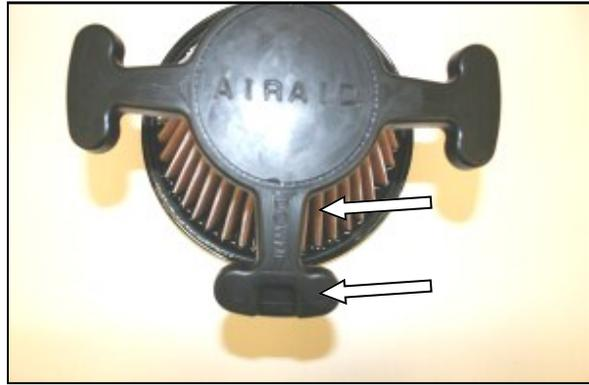
4. Locate the word "Down" on the filter and notice that there is a notch below it. It is important to locate this notch in the correct location in the bottom of the factory airbox.
