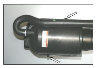
1. Disconnect the Negative Battery Cable. Unlatch the two factory clips on each side of the airbox and then remove the airbox lid.
