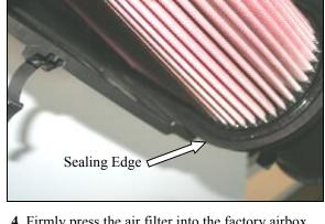
**4.** Firmly press the air filter into the factory airbox. Make sure that the sealing edge is fully seated and flush with the edge all the way around the airbox.
