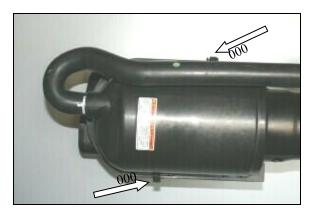
**6.** Reinstall the factory airbox lid and re-latch the two factory clips. **Double check your work!**
