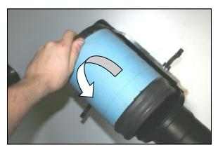
2. Remove the factory air filter by gently prying it towards the passenger side of the airbox, and then lifting it straight up.
