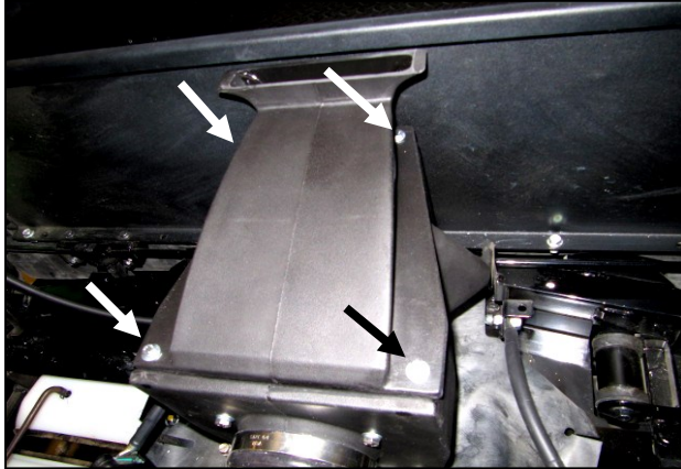
14. Complete the assembly by installing the Air Box Top (#2) onto the Cold Air Box using four 1/4-20 x 1" bolts (#7), 1/4" lock washers (#10), and 1/4" Flat washers (#9).
