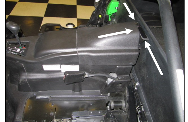
15. Reinstall the factory covers in the reverse order of removal. Reconnect the battery terminal and reinstall the seats. Notice that the Air inlet is now located outside of the engine cover.
