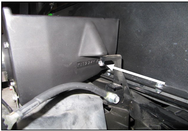
11. Secure the rear half of the of the CAB assembly to the Horizontal brackets using two 1/4-20 x 5/8" bolts (#6), 1/4" lock washers , and 1/4" Flat washers.
