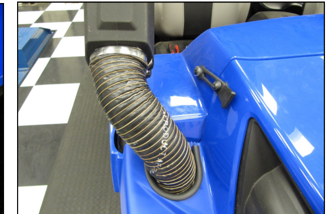
15. Align the Snorkel and Ducting and verify the opening and closing action of the hood is not adversely effected. Tighten all of the Clamp bolts when done.
