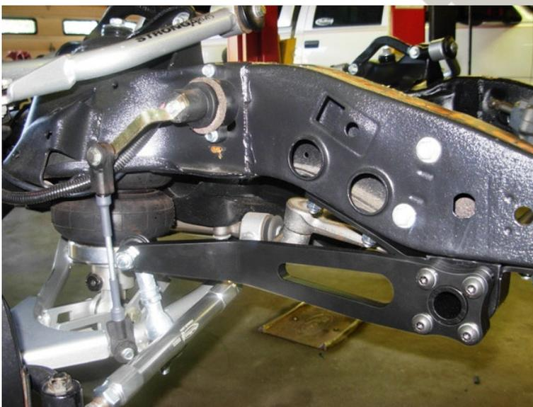
3. Two of the three holes on the front of the bracket will align with existing holes. The outer hole must be drilled to 7/16".
