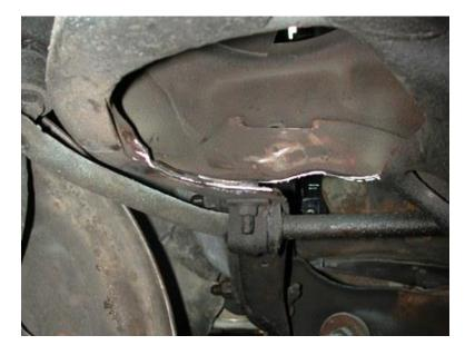
4. After double checking Shockwave clearance grind all edges smooth and paint exposed metal.
