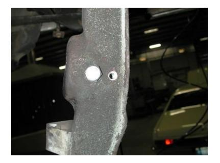
9. Drill the factory shock hole in the lower control out with a 1/2" bit.
