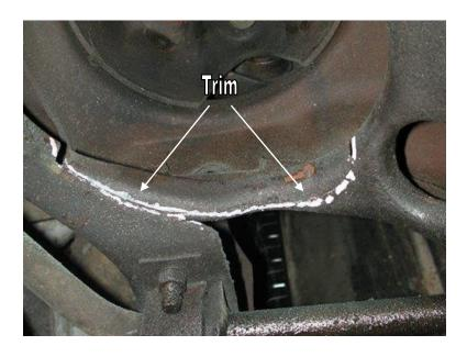
3. The front and outside lip of the coil spring pocket must be trimmed to allow clearance for the Shockwave. This is best done with a die grinder and a cut off wheel.
