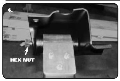
**4.** Bolt the **LARGE BUSHING END** of the Composite Leaf Spring into the OEM front leaf spring mount using a 1/2"-13 x 5" Hex Bolt and 1/2"-13 Nylok Nut. The Bolt must be installed with the threads pointing to the **OUTSIDE** of the car. Diagram #4 is the correct orientation.
