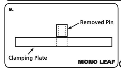
**9.** The kit contains 4 Clamping Plates that are all the same. For a Mono Leaf installation, the center pin will need to be removed from **2** of the plates. The pin can be knocked out with a hammer and punch.
