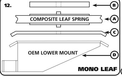
Diagrams 10, 11, & 12 will be used to aid in the installation of the Clamping Plates on a Mono Leaf Differential.
