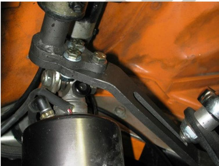
4. Position the axle to ride height, 14.5" from eye to eye on the Shockwaves/Coilovers. Then position the sway bar so that the arms are level to the ground.
