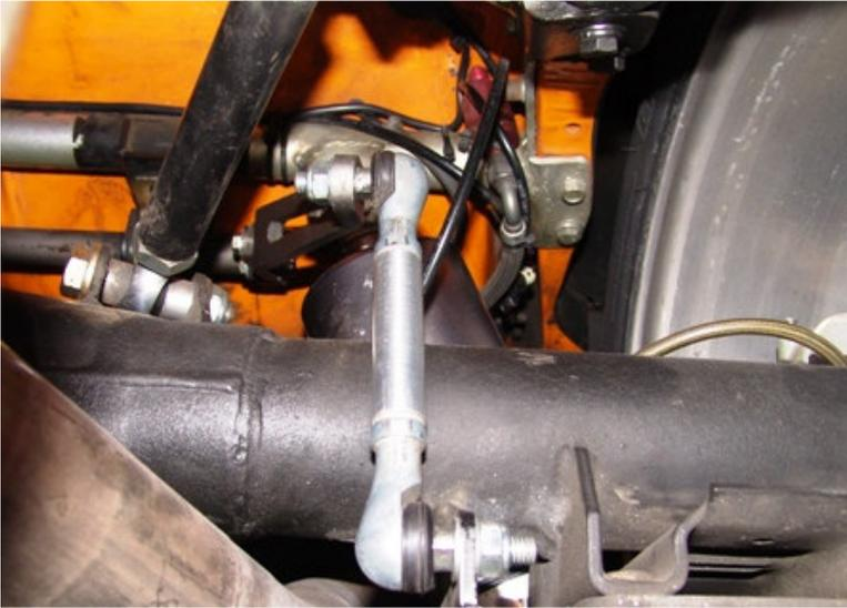
7. Swing the axle through full suspension travel checking sway bar clearance and ensuring that the PosiLinks do not bind.
