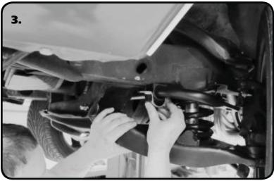
**3.** Install Bushing Straps Over the Poly Sway-Bar Bushings.
