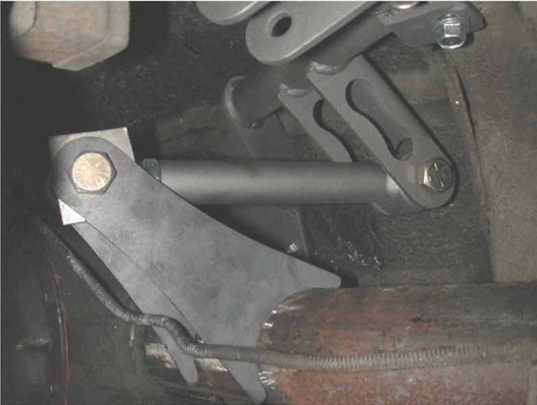
10. Bolt the upper bar to the cradle using a 5/8" x 2 3/4" bolt and Nyloc nut.
