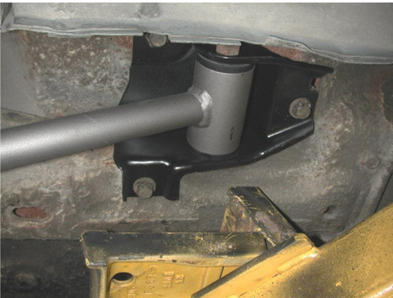
3. Fasten the large end of the lower bar to the factory leaf spring hanger using the factory hardware. Then reattach the hanger to the car. These two larger bushings are polyurethane and are lubricated at the factory. Future lubrication can be done with any non petroleum based lubricant such as lithium or silicone.
