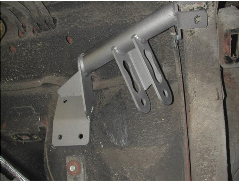
8. Using the cradle as a template, drill four 3/8" holes in the floor pan.
