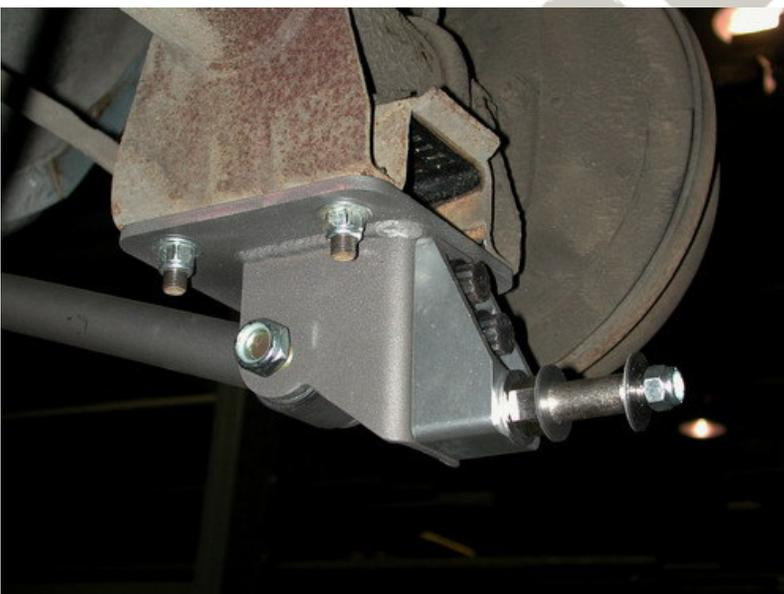
4. Bolt the lower bar axle mount to the leaf spring pad using the factory studs and U-bolt. New 7/16" Nyloc nuts are supplied.
