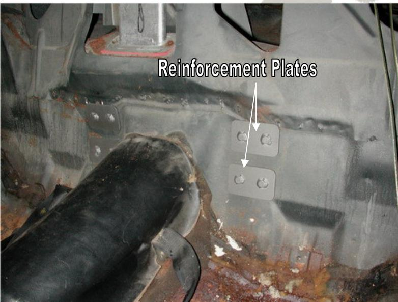
9. From the inside of the car drop the reinforcement plates through these holes. Secure the assembly with 4 3/8" Nyloc nuts and flat washers. You may need to flatten part of the seam just above the top two holes.
