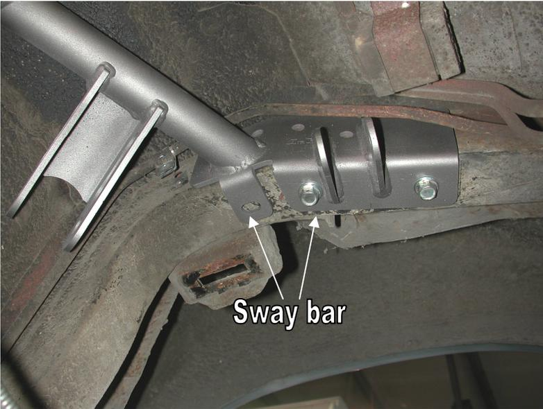
7. Raise the upper cradle into position against the body and clamp in place. The contour of the plate will match the contour of the body. On cars that came with a factory sway bar the two forward holes on the bottom will already be there. The rest of the holes must be drilled with a 5/16" bit. Use the 3/8" x 1" thread forming bolts to secure the assembly.
