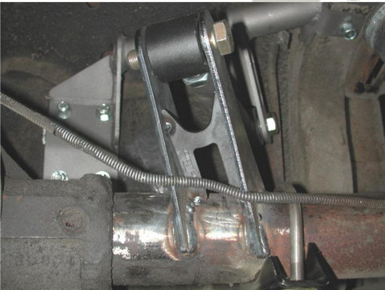
16. Once everything is double-checked the tabs can be tack-welded into place. Then tack in the axle tab brace between the two tabs.
