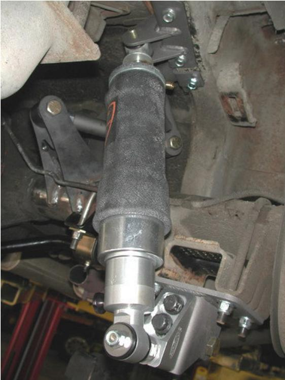
19. Apply thread sealant to an elbow air fitting and screw it into the top of the Shockwave.
