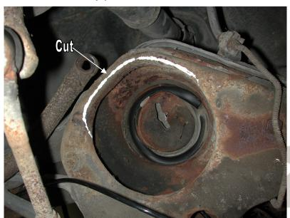
3. The outer lip of the coil spring pocket must be removed for air spring clearance. This is best done with a cut off wheel or plasma cutter. Grind smooth when finished.
