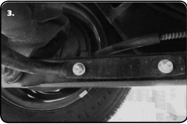
**3.** Slide the bar in Place with the LOW part of the bar down. Install a 7/16" washer on one of the 7/16"-14 x 3" Bolts and install one in each Front Hole to help hold it in place. Swing the SwayBar into position and insert the Rear Bolt/Washer. Tighten Hardware.
