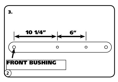
**1.** Some Cars have a Small Hole at the Front Bolt Location, if yours has it, Drill it out with a 7/16" Drill Bit and then Mark a Hole 6" towards the rear of the Car and Drill. If your Car has no Holes, Measure back 10 1/4" from the center of the Front Bushing and make a mark centered top to bottom. Next measure back 6" from your first mark and Mark the Second Hole centered Top to Bottom. Drill the Locations with a 7/16" Drill Bit going through both Sides of the Arm. Repeat for both Arms.
