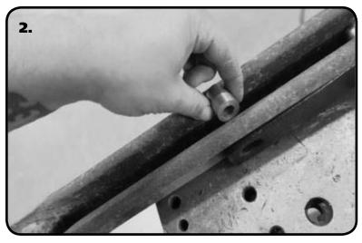
**2.** Insert the Supplied Spacer into the inside of the Control Arm at the Hole Locations. These Spacers will get Clamped in place by the Mounting Hardware after the SwayBar is installed. These can be welded in place if desired.
