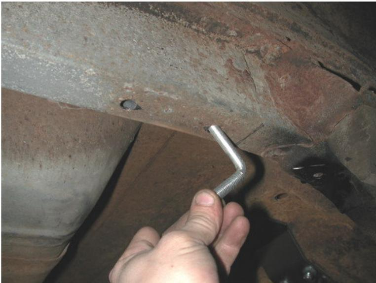
8. Remove the crossmember and drop the 3/8" U-bolt through the holes. Reinstall crossmember and tighten with 3/8" nylocs and flat washers.
