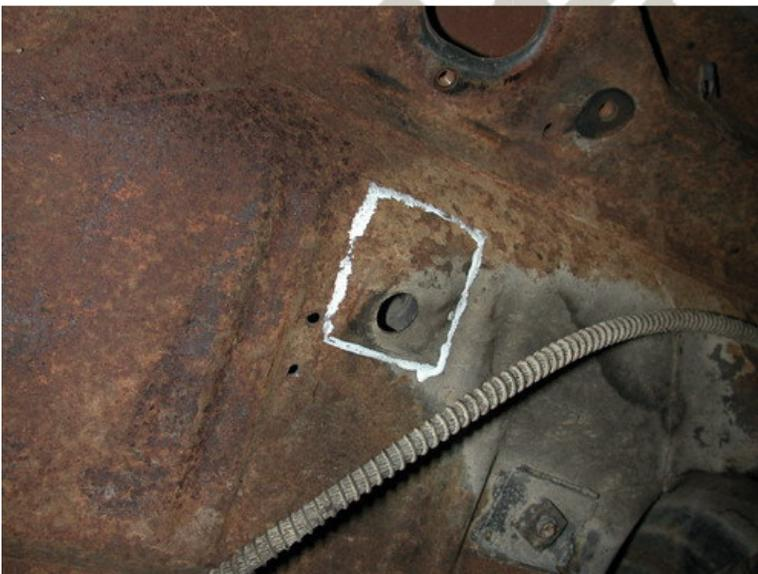
2. Remove the gas tank sending unit wire from the tank and pull it into the trunk.
