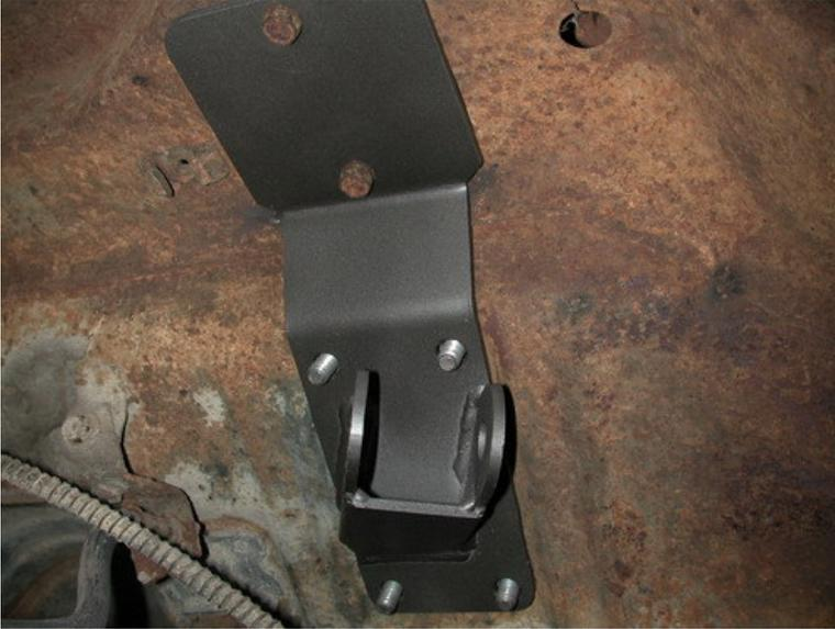
4. The upper bar mount will bolt to the bottom of the car using the factory shock bolts and locates off the factory shock mount.
