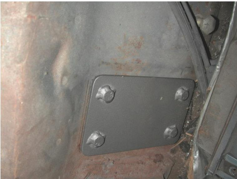
6. The upper bar bolt plate can be dropped into place from the trunk. The bracket will be clamped into place using 3/8" nylocs and flat washers.
