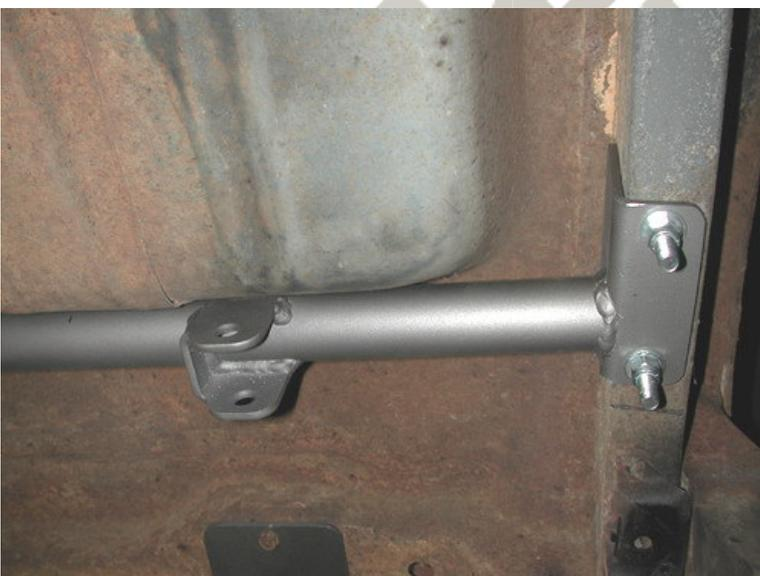
7. Lower the axle enough to slide the upper crossmember into place. The frame is wider towards the rear of the car as is the crossmember. Push it forward until it is tight between the frame rails, but make sure it is square. Drill two holes with a 7/16" drill bit.
