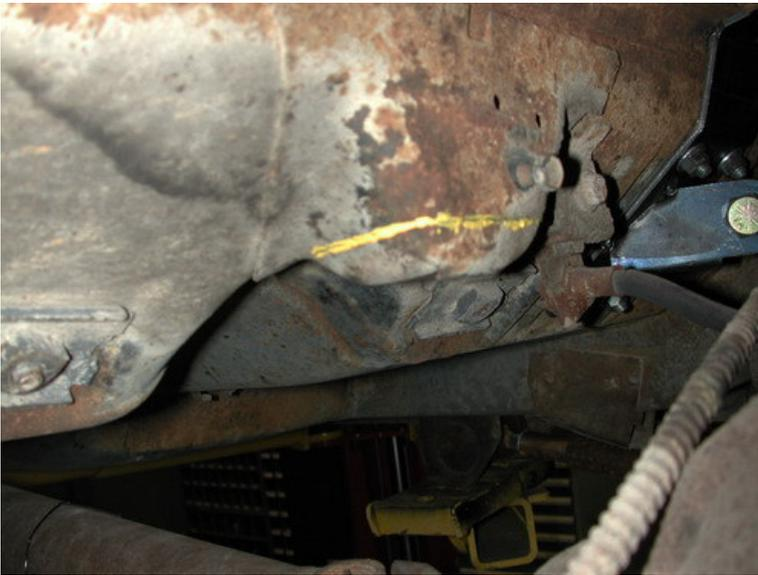
1. The pinion snubber mount must be cut on the line shown in the picture. This allows more clearance of the pinion for maximum drop.
