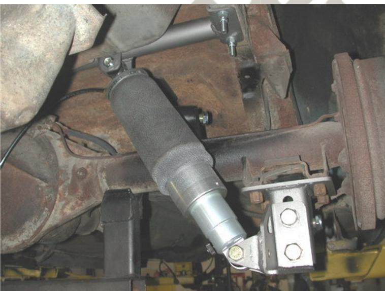
20. Apply thread sealant the air fitting and screw it into the top of the Shockwave.
