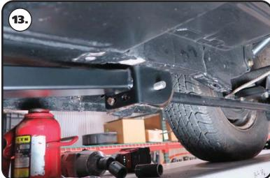
**13.** Tighten the bolt down in **Step 11** This will tighten the connector against the leaf spring mount.
