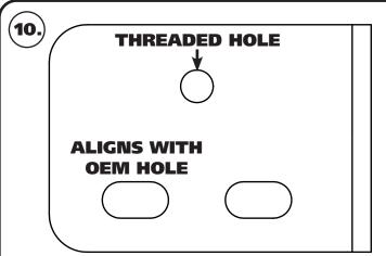
**10.** The top hole is a "blind" hole. A template is provided on **Page 10** to help with drilling of this hole. Drill the holes with a 7/16" drill bit.
