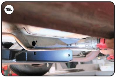
**15.** Loosen the front bolt at the leaf spring mount to allow the front of the connector to drop down. Pull the front of the connector down to gain access to the sides of the frame rail. Drill the 2 OUTER frame rail holes out to 3/4". We use a unibit to drill the holes.
