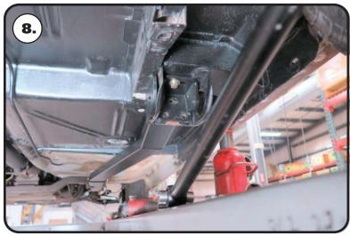
**8.** If installing this kit with the Ridetech 4 link, we recommend doing one side at a time. This will help hold the differential in place while installing the connectors. Disconnect the front of the lower bar from the bar mount. The (3) front bolts will also need to be removed.
