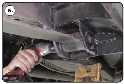
**6.** Remove the OEM leaf spring hardware from the front of the leaf spring. Retain the leaf spring hardware for reassembly.
