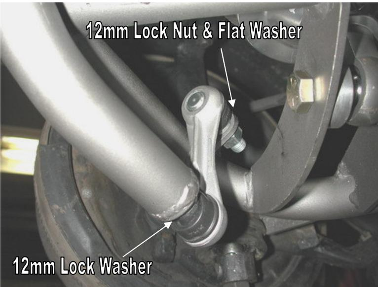
9. The other end of the PosiLink will attach to the tab on the StrongArm using a 12mm flat washer and locking nut.
