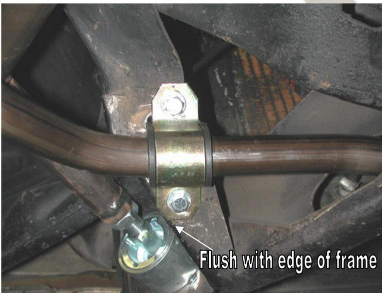
4. Adjust the frame bracket so that the corner of the bracket is flush with the outside of the frame rail.
