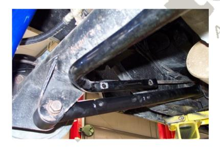
4. Attach to rear of the lower StrongArm to the frame using the factory hardware.
