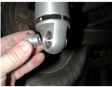
9. Install the aluminum spacers into the upper and lower eyes of the shock.
