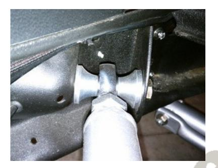
1. The length of the upper bar should be set from the factory at 11.125" center to center. Ensure that the jam nut is tight.
