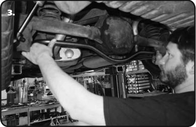
**3.** Slide the bar in Place with the LOW part of the bar down. Install a 3/8" washer on one of the M10-1.5 x 70mm Bolts and install one in each Front Hole to help hold it in place. Swing the SwayBar into position and insert the Rear Bolt/Washer. Tighten Hardware.
