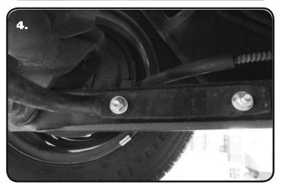
**4.** Install a 3/8" washer on one of the M10-1.5 x 70mm Bolts and install one in each Front Hole to help hold it in place. Swing the SwayBar into position and insert the Rear Bolt/ Washer. Tighten Hardware.
