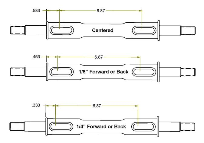
These Strong Arms come equipped with a changeable caster slug setup. This allows you to add or remove caster from the front suspension, if desired. The caster slugs that come in the kit are setup to put the control arm in the centered position, which is approximately 5 degrees of caster. The caster slugs allow you to add or remove caster without having to use a stack of shims. If more or less caster is desired, optional caster slugs can be purchased from your Ridetech dealer or Ridetech.
