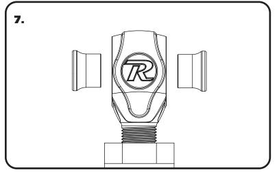
**7.** Assemble the Panhard bar. Install a 3/4"-16 Jam Nut on the shank of the R-Joint end. Thread the R-Joint end into the bar. Set the Center to Center dimension of the panhard bar to 36". Install the R-joint Spacers into the center pivot ball of the R-Joint. Insert the small end of the spacer into the center ball, push it in until it stops.
