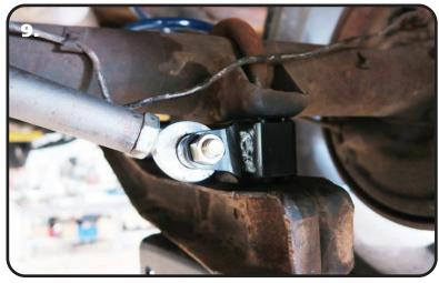
**8.** Install the panhard bar in the frame mount. Install a 5/8" Flat Washer on a 5/8"-18 x 3 1/2" Hex Bolt and insert it through the Mount, Spacers and Panhard bar. With the Bolt installed, install a 5/8" Flat Washer on the threads followed by a 5/8"-18 Nylok Nut.
