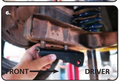
**6.** If you purchase the StreetGrip Shock Kit, install the lower mount at this time. The Mounts are installed on the U-Bolts, on the bottom side of the trailing arm. The shock mounting hole should be positioned with the hole to the front and to the inside of the truck. Once the Mount is installed, install a 3/4" Flat Washer and 3/4"-16 Nylok Nut on each leg of the U-Bolts. Tighten the Nylok Nuts to 350ftlbs.
