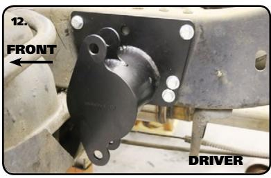
12. The Bar Mounts bolt in place of the OEM front leaf spring mount. There is a Driver and Passenger Mount. Image 12 shows the Driver Mount. The Tabs are to the FRONT of tube. Install a 7/16" Flat Washer on (6) 7/16" x 1 1/4" Bolts. Hold the Mount in place and insert the bolts/washer through the mount and frame. Install a 7/16" Flat Washer and 7/16" Nylok Nut on each bolt sticking through the frame and tighten to 50 ftlbs. Repeat on the other side.
