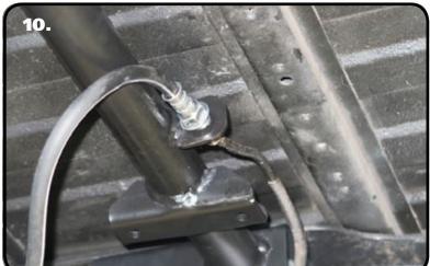
**10.** Attach the rubber brake line to the Upper Cross Member using the OEM clip. You may have to tweak the steel brake line to reposition it to thread into the rubber brake line. Thread the steel brake line into the rubber brake line and tighten.
