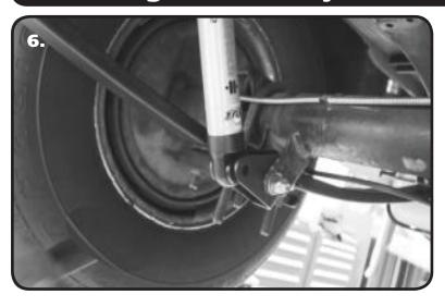
6. Slide the bottom of the Shock into the new Mount. Line up the Shock with the Mounting Hole in the Lower Mount. You may need to jack up the differential to get the holes lined up. Install a 1/2" Flat Washer on a 1/2"-20 x 2 1/4" Bolt. Insert the Bolt/Washer into the Mount/Shock. Install a 1/2"-20 THIN Nylok Nut on the threads sticking through. Do this for both sides and tighten hardware.
