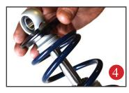
Slide the Derlin washer over the spring, Next slide the upper spring mount (90002222) over eyelet as seen in figure 4.
