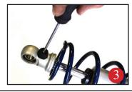
Before the upper spring mount can be installed screw the adjuster knob on the upper eye mount to the firmest setting (clockwise) as seen in figure 3. Then remove the knob.
