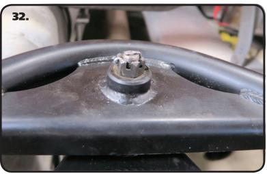
**32.** Torque the ball joint nut to 50 ftlbs. Verify if the hole in the ball joint pin aligns with any of the slots of the castle nut. Tighten the castle nut to align them. DO NOT LOOSEN THE CASTLE NUT. The thread the grease zerk into the ball joint and grease it.
