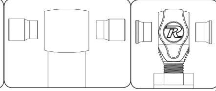
New R-Joints will be quite stiff (75-90 in/lbs breakaway torque) until they "break in" after a few miles of use. After the break in period they will move much more freely. Because the composite bearing race contains self lubricating ingredients, no additional lubrication is needed or desired. Any additional lubrication will only serve to attract more dirt and debris to the R-Joint and actually shorten its life.
