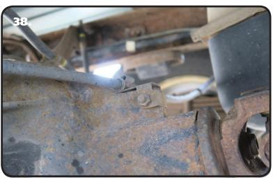
**38.** On some years, the emergency brake cable mounting will need to be modified for clearance. If your cable mount on the snout of the differential looks like **Image 38**, no changes will be needed. If it looks like **Image 39**, the mount will need to be flipped around.
