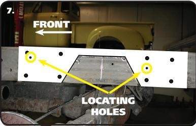
**7.** Use the supplied Template to mark the cut lines on the frame. Center Punch the "\(\psi\)" in the corners of the cut area.
