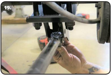
**19.** Insert the Rear Lower Bar R-Joint into the Lower Axle Bracket. Line up the through hole of the R-Joint with the of holes of the Axle Bracket.
