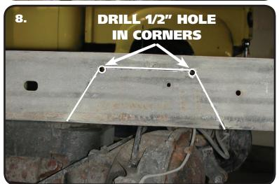
**8.** Drill out the two corners with a ½" drill bit. This will give the cut a round edge and eliminate the possibility for stress fractures. Then cut the notch with a saw-z-all, cutoff wheel, or plasma cutter. Grind all edges smooth. Check the inside of the frame for wires or lines before drilling or cutting.
