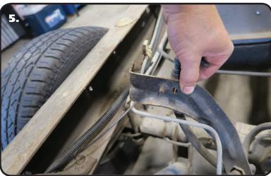
**5.** Unbolt the brake line bracket from the inside of the driver side frame rail.
