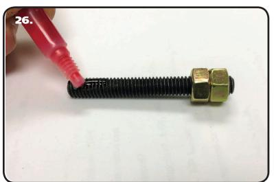
26. The 9 OEM bolts that were removed from the top of the differential cover will be replaced with M8-1.25 x 50mm Studs. These Studs and the nuts used to install them are supplied in the Hardware Bag labeled "Upper Wishbone Differential Mount". Thread the (2) M8-1.25 Hex Nuts on one of the studs. Using (2) wrenches, tighten the nuts against each other locking them together. Apply Red Loctite to the other end of the stud.
