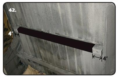
**42.** Trimming of the bed brace that is in between the wheel wells is necessary to clear the c-notches and wishbone. We cut ours with a diegrinder and cut off wheel. **Image 42** illustrates the bed brace cut out. The cut starts 4" from the end of the brace and runs all the way across leaving 4" on the other end. It needs to be cut even with the flange that attaches the brace to the bed floor.
