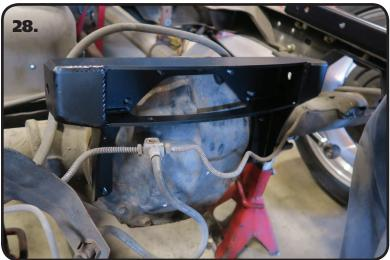
**28.** Position the Axle Bracket/Wishbone in place with the wishbone to the front of the truck. Line up the (9) holes in the axle bracket with the (9) sutds of the Differential.
