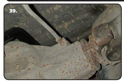
**39.** If your emergency brake cable mount looks like **Image 39**, the mount will need to be flipped around. Start by removing the nut from the attaching bolt. Next, remove the bolt to detach the mount from the snout of the differential.
