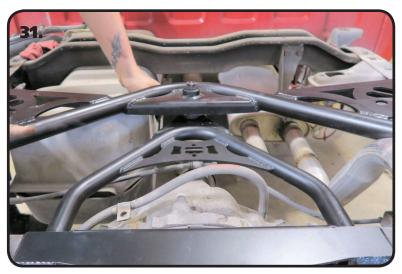
**31.** Insert the ball joint pin into the opening of the upper bridge. Push it up in the hole and install the castle nut supplied in the kit.
