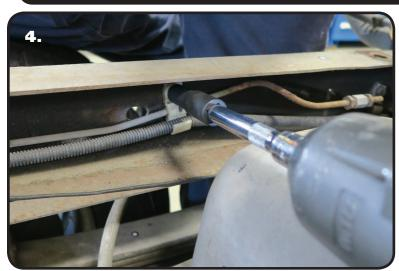
**4.** The brake line/wire clamp will need to be removed from the inside of the driver side frame rail. This will allow you to move it out of the way when cutting the frame for the c-notch.
