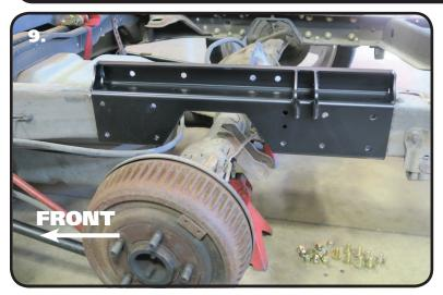
**9.** Slip the C-Notch over the frame rail. Use the C-Notch as a template to drill the (10) holes in the side of the frame. Use a 7/16" drill bit to drill the holes. Install a 7/16" Flat Washer on each of (10) 7/16"-14 x 1 1/4" Bolts. Insert a bolt/washer in each hole. Install a 7/16" Flat Washer and 7/16"-14 Nylok Nut on the threads of each bolt/washer and tighten. Torque the hardware to 50 ftlbs.
