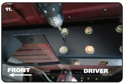
**11.** Drill out the small rear locating hole to 5/16". Also, remove the nut from the 7/16" Bolt above the small hole. Install a 5/16" Flat Washer on (1) 5/16"-18 x 1 1/4" bolt and insert into the drilled hole.
