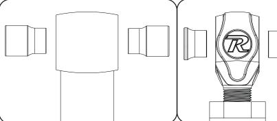
New R-Joints will be quite stiff (75-90 in/lbs breakaway torque) until they "break in" after a few miles of use. After the break in period they will move much more freely. Because the composite bearing race contains self lubricating ingredients, no additional lubrication is needed or desired. Any additional lubrication will only serve to attract more dirt and debris to the R-Joint and actually shorten its life.
