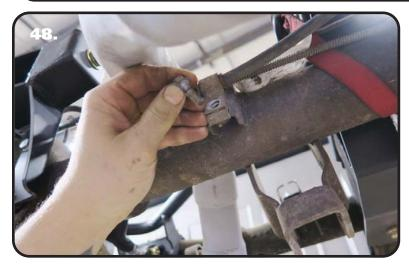
**48. Steps 48-52** cover the emergency brake cable relocation. The cables need to be relocated to gain Shockwave/CoilOver clearance. Start by removing the bolt that clamps the passenger side cable to the driver side axle tube. Spread out the clamp to remove it from the cable. Retain the clamp, it will be reinstalled.
