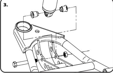
**3.** Raise the lower arm up to the CoilOver and bolt them together using the 1/2" x 3 1/2" bolt, flat washer, and nylok supplied w/ the lower arms. An aluminum spacer will be on each side of the bearing. Torque to 75 ftbs.
