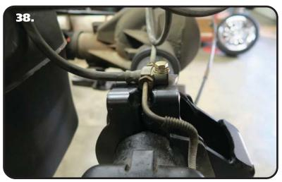
**38.** If your truck required the brake line bracket to be cutoff the axle tube, reattach it to the top of the panhard mount. Use the 5/16"-24 x 1 " bolt, 5/16" split lock washer, & 5/16" SAE flat washer that's supplied in the kit.
