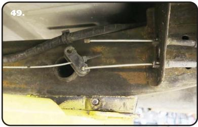
**49.** Disconnect the top cable from the cable yoke. This can be done by twisting the top of the yoke to the rear enough to get the cable out.
