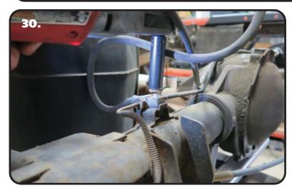
**30.** Remove the bolt that attaches the brake hose to the bracket. This will allow you to move the brake line out of the way to cut the bracket off the axle tube.
