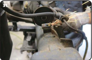
**31.** We used a die-grinder with a cutoff wheel to cut the brake line bracket off the axle tube. Be careful to not cut into the axle tube.
