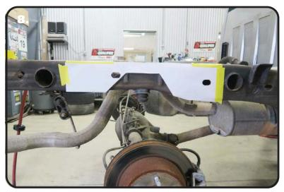
**6.** To allow maximum drop on this truck, the frame must be notched. The template for the notch will locate off of the 2 large oval holes. Use the supplied "C" Notch template to mark out the frame for cutting. Before cutting out the frame, support the frame in front of and behind the "C" Notch area. We suggest doing one side at a time. The tall end of the template is located to the front of the truck
