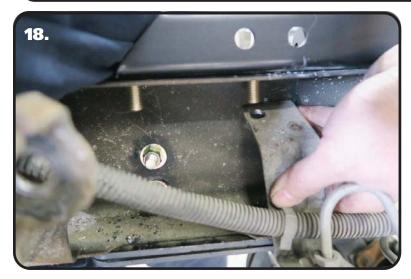
**18.** Remove the nut and washer from the 2nd from rear top bolt of the driver side c-notch. Install the brake line bracket on the bolt and reinstall the nut and washer. If your truck is 2001 and newer, tighten the top and bottom c-notch hardware to 50 ftlbs then skip to step 20. If you have a 1999 - 2000, proceed to step 19.
