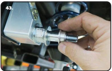
**43.** The Shock Stud requires spacers that are .400" long (90002067). Install a 5/8" ID 90002067 spacer **(Small side towards shock body)** onto the lower Shock Stud. Slide the bottom of the Shock onto the Stud. Install a second 5/8" ID 90002067 Spacer onto the Stud **(small side towards shock)**. You may need to jack the rear end up to Slide the Shock onto the Stud.
