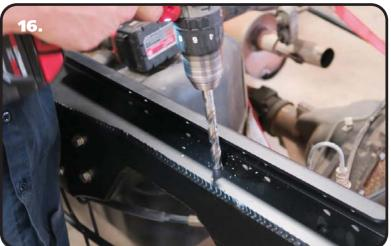
**16.** Use a 7/16" drill bit to drill the remaining holes in the top and bottom of the frame. Install a 7/16" Flat Washer on the remaining 7/16" x 1 1/4" Bolts. Insert bolt/washers in the drilled holes of the c-notch. Install a 7/16" Flat washer and 7/16" Nylok Nut on the threads sticking through the c-notch/frame. DO NOT TIGHTEN.
