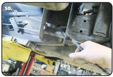
**50.** Disengage the cable from the frame mount and pull it out. The cable runs over the top of the axle from the factory, it needs to be pulled out and rerouted under the axle. Reroute the cable under the axle and reinsert in into the frame mount and connect to the yoke.
