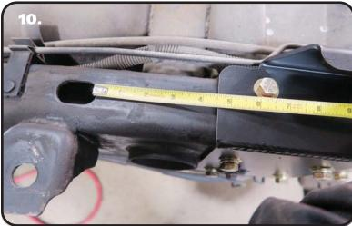
**10.** The front edge of the c-notch should be 4 1/2" from the oval hole in front of it. Trim the opening to move the c-notch forward or backward to achieve 4 1/2".
