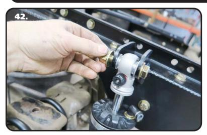
**42.** Insert the 1/2" ID Shock Bearing Spacers into the Bearing of the ShockWave/CoilOver. Install a 1/2" Flat Washer on a 1/2"-13 x 2 3/4" Bolts. Insert the top of the shock into the shock mount on the c-notch with the adjusting knob to the outside. Line up the holes and insert the bolt/washer. Install a 1/2" Flat Washer and 1/2"-13 Nylok Nut on the threads and tighten to 50 ftlbs.
