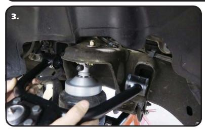
**3.** The Driver and Passenger Control Arms are identical. Insert the Control Arm into the OEM frame mount with the balljoint stud pointing down. The Gussets of the Balljoint Plate should also point down.
