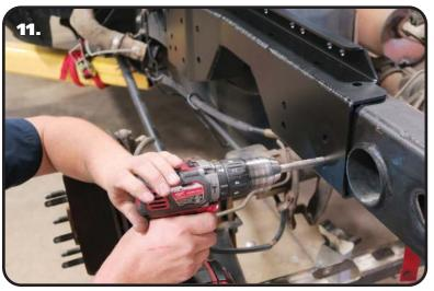
**11.** Use a 7/16" Drill bit to drill the holes in the side of the frame. DO NOT DRILL THE HOLES WHERE THE EMERGENCY BRAKE CABLE BRACKET IS BOLTED, OR THE TOP AND BOTTOM OF THE C-NOTCH. There are 10 holes in the side that need to be drilled.
