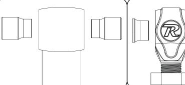
New R-Joints will be quite stiff (75-90 in/lbs breakaway torque) until they "break in" after a few miles of use. After the break in period they will move much more freely. Because the composite bearing race contains self lubricating ingredients, no additional lubrication is needed or desired. Any additional lubrication will only serve to attract more dirt and debris to the R-Joint and actually shorten its life.
