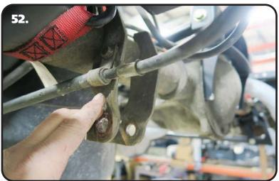
**52.** The Driver side emergency brake cable only requires the clamp be moved on the cable. Remove the attaching bolt and spread out the clamp enough to allow it to be moved. Move the clamp from the metal area to the rear edge of the plastic sheath. The rear edge of the clamp will line up with the rear edge of the sheath. Use the OEM bolt to reattach it.
