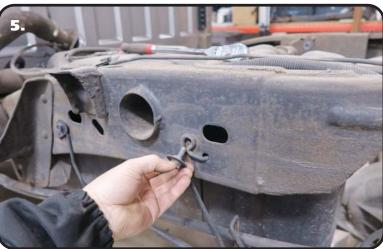
**5.** Unbolt the emergency brake cable bracket from the driver side frame rail. It is located between the axle and the front leaf spring hanger. Retain the hardware for reassembly.
