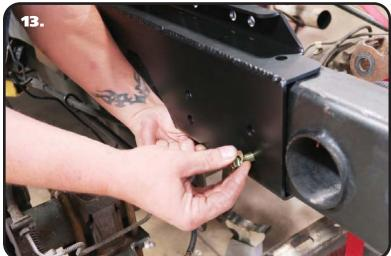
**13.** Install a 7/16" lock washer, & 7/16" flat washer on (4) 7/16" x 1 1/4" Bolts. Install them in the rear 4 holes of the c-notch. Install a 7/16" flat washer and 7/16" nylok nut on each bolt sticking through the frame. Repeat on the other side.
