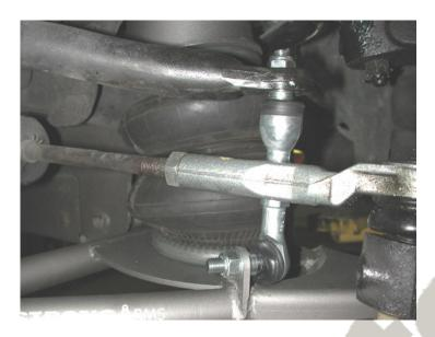
1. Apply lubricant to the poly bushing and slide it over the sway bar. Using the frame brackets supplied bolt the sway bar to the frame. Do not tighten the bolts yet.
