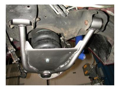
1. After removing the factory lower control arm, clean the bushing mounting surfaces on the frame and lubricate with Lithium grease.
