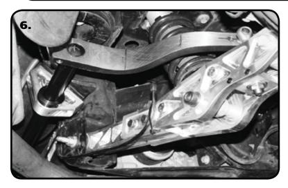
**6.** The PosiLink can be used to get the arms clocked the same. Install one Arm on the Drivers Side and rotate it up and down until you can insert the PosiLink in the center hole. On the Passenger Side, install the arm on the Sway Bar. Try to insert the PosiLink in the center hole. Remove the Arm from the Splines and move it one Tooth at a time, reinstalling the arm until the PosiLink will go in the center hole easily.
