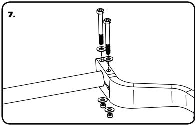
**7.** After the arms are installed, insert (2) 5/16" x 2 3/4" bolts with a 5/16" washer on each, through the Clamping Holes in the Arms. Install a 5/16" Flatwasher and 3/8" Nylok on the Bolt and Torque to 25 ftlbs. It will be necessary to torque each bolt multiple times.
