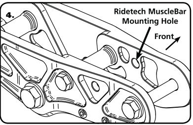
**4.** Use Diagram 5 to determine the correct PosiLink assembly for each side. Attach the PosiLinks to the StrongArm in the location shown in Diagram 4. Install 3/8" Flatwasher and 10mm Nylok nut on each PosiLink and tighten down.
