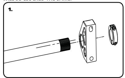
**1.** Install both Bushing Mounts onto the Splined Bar with the Flange side of the Inner Bushing facing out. With the Bushing Mount slid onto the bar, install the Locking Ring, but do not tighten.
