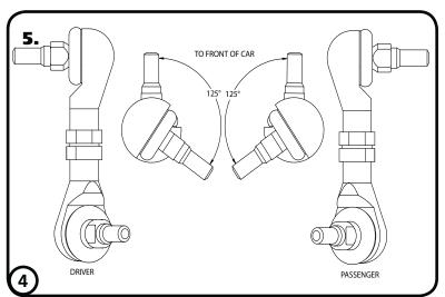
**5.** Diagram 5 shows the difference between the Driver and Passenger PosiLinks.
