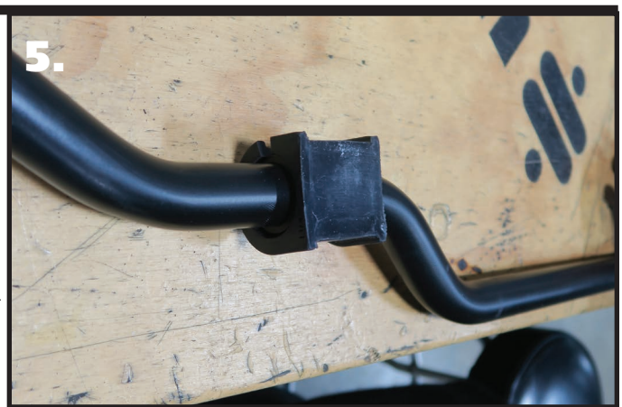
5. Open the SwayBar Bushing at the split and slide it OVER the Delrin Liner. Do this on both Delrin Liners.
