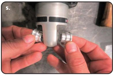
**5.** Install the 1/2" I.D. bearing spacers into bearing in the shock body. These spacers have a through hole that is 1/2" diameter. The small diameter of the spacers will insert into the shock bearing.
