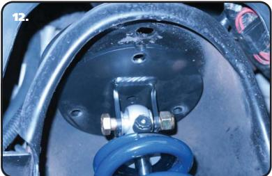
**12.** The Upper Mount needs to be positioned with the NOTCH toward the wheel. The shock adjuster knob should also be toward the wheel.
