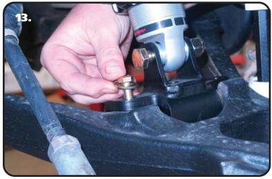
**13.** Align the mounting holes of the lower mount with the OEM shock mounting holes in the lower control arm. Install a 5/16" flat washer on each of (2) 5/16"-24 x 2 1/4" hex bolts. Insert the bolts/washers in the aligned holes of the lower mount and control arm.
