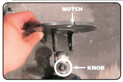
**8.** Attach the Upper Mount to the shock eye. The mount needs to be attached to the eyelet so that the notch is on the same side as the adjuster knob.
