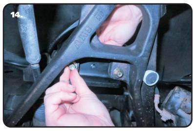
**14.** Install a 5/16" flat washer and 5/16"-24 nylok nut on the threads of the bolts sticking through the lower control arm. Torque the hardware to 29 ftlbs.
