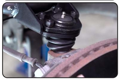
**6.** Insert the pin of the upper balljoint into the spindle.
