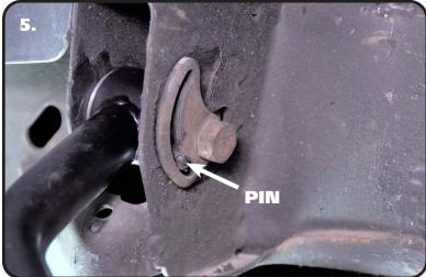
**5.** Reinstall the OEM adjuster bolts. Make sure the PINS in the frame are located in the slots of the adjuster. Set the adjuster back to the marks made during disassembly and torque to 140 ftlbs.
