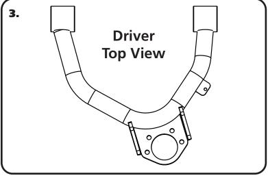
**3.** The upper control arm is attached to the factory mount using the factory hardware. The driver side arm is shown in **Figure "3"**. The ball joint on the arm is oriented to the rear of the truck. The brake line tab on the control arm will be to the REAR of the control arm.
