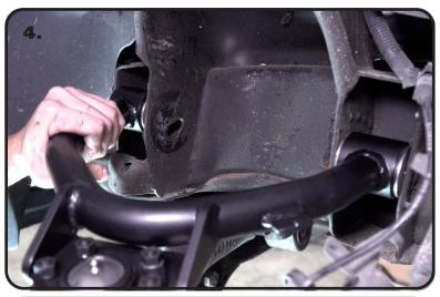
**4.** The upper control arm is attached in the factory mount using factory hardware. The driver side arm is shown in **Figure "3 & 4"**. Line up the through holes of the bushings with the OEM slots.
