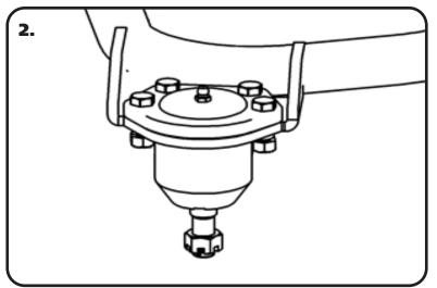
**2.** Install the ball joints into the upper control arm with the hardware supplied with the ball joint. The upper ball joint goes in from the top side of the control arm. The gussets on the ball joint plate point up. Torque the hardware to 29 ftlbs.
