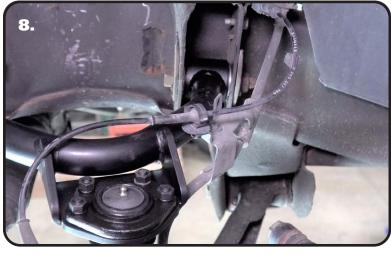
**8.** Attach the brake line bracket to the new upper control arm using the supplied thread forming bolts. Align the bracket with the tab on the control arm. Attach it using the thread forming bolts supplied with the kit. These can be threaded in using a ratchet. Put downward pressure on the bolt while turning them. Torque them to 15 inlbs.
