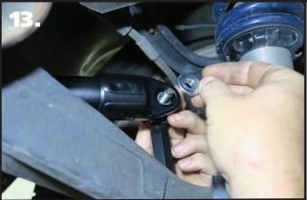
**13.** Install a 2nd t-bushing with the small diameter into the swaybar.
