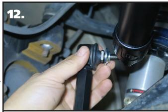
**12.** Insert the 90 degree end link/t-bushing into the swaybar end with the threads pointing toward the center of the truck.
