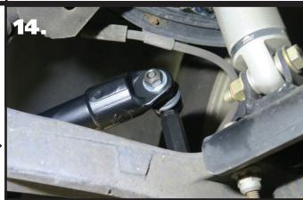
**14.** Install the nut that came supplied on the end and torque. Do this for both sides.
