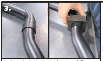
**3.** Open the Delrin Liner at the split and slip it over the SwayBar. Position it in the area that the bushing will ride based on the location of the stock swaybar. Do this on both ends of the swaybar. Next, open the SwayBar Bushing at the split and slide it **OVER** the Delrin Liner. Do this on both Delrin Liners.
