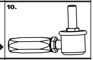
**10.** Use 2 wrenches to lock the jam nut against the spacer. Your assembly should look like **Diagram 10**.
