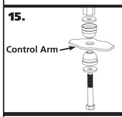
**15.** Install the End Links using **Diagram 15** as a reference. The supplied 7/16"-20 x 3" bolt is used to attach the end links to the control arm. Install both end links before tightening the end link hardware. Tighten the bolt until it bottoms out.
