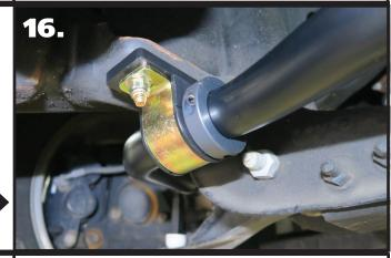
**16.** Install the stop rings against the swaybar bushing. The stop rings will go against the inner side of the bushing. Take the stop rings apart and reassemble them against the bushing and tighten.
