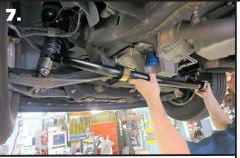
7. Slide the swaybar into position with the center of the bar being the lowest point. Slip the swaybar bushing straps onto the studs of the mounting plates.
