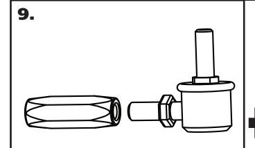
**9.** The swaybar end links will need to be partially assembled before they can be installed. Using your fingers, thread the jam nut all the way on until it stops. Thread the spacer onto the stud until it stops against the jam nut.
