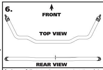
**6. Image 6** illustrates the correct orientation of the swaybar. With the arms level, the center of the bar should be lower than the arms.
