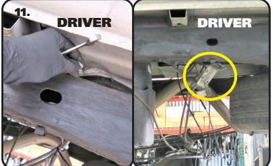
**10.** Remove the ABS sensors from the axle tubes on driver and passenger side. DRIVER SIDE IS SHOWN IN **IMAGE 10**.
