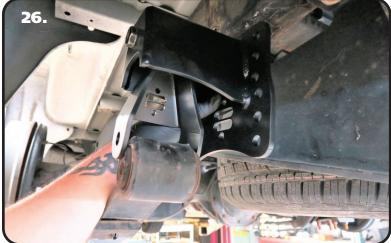
**26.** Raise the rear of the leaf spring up until it lines up with the rear shackle. You may have to jack up the rear differential. Install the OEM hardware that was removed earlier. Repeat on the second spring. Do not tighten the hardware at this time.
