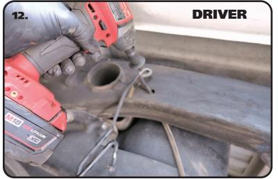
**12.** Remove the emergency brake cable holder from the driver side frame rail. Again, this bracket will be reinstalled later.
