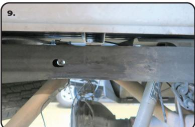
**9.** We recommend grinding the remaining weld down until it is smooth. Paint the exposed metal to keep it from rusting.
