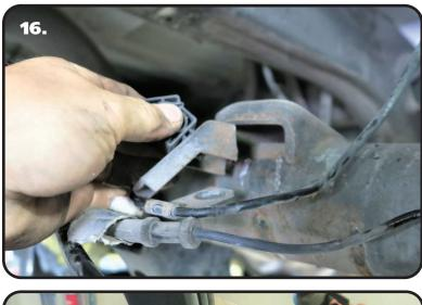
**16. Image 16** illustrates the bracket cut off. Again, we use a saw-z-all to cut it off.
