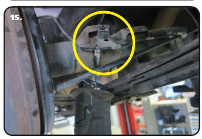
**13.** Remove the bolt from the brake line retainer. The brake line retainer bolts to the bracket that is on the rear side of the leaf spring perch. Remove these from both sides of the axle. These will be reinstalled later.
