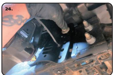
**24.** Determine the set of holes that you are going to be using to attach the hanger. The Hanger is bolted to the frame in the OEM location with the open side of the shackle to the front of the truck. The REAR UPPER hole reuses the OEM bolt that was removed earlier. Install the OEM bolt in the rear upper hole. This will help hold the hanger while inserting the remaining bolts.
