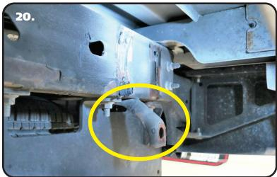
**20.** The OEM leaf spring hanger includes a second bracket that is riveted to the bottom of the frame. Again, cut a " + " in the head of the rivet and chisel it off. After removing the head of the rivet, drive it out of the frame/ bracket with a punch. Repeat steps 19-20 on the second hanger.
