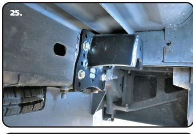
**25.** Install a 7/16" flat washer on each of (3) 7/16"-14 x 1 1/4" bolts. Align the correct holes of the hanger with the OEM holes in the frame. Install a bolt/washer in each one. Install a 7/16" flat washer and 7/16"-14 nylok nut on the threads of the bolts that are sticking through the frame. Torque the hardware to 70 ftlbs.
