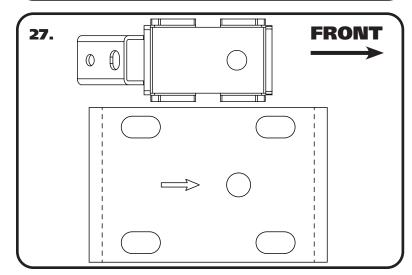
**27.** The Flip Kit has the locating holes offset to center the wheel in the wheel opening. **Image 27** illustrates a top view of the Flip Bracket and the Leaf Spring Plate. Notice the CENTER Hole is offset to the FRONT of the truck. The Flip Bracket has a brake line tab that will need to be positioned to the rear of the truck. The ARROW in the plate needs to point to the front of the truck.
