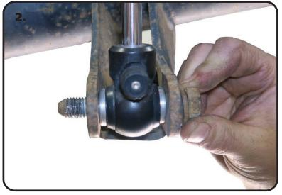
**1.** Install the BODY of the shock in the OEM frame mount using the OEM hardware.
