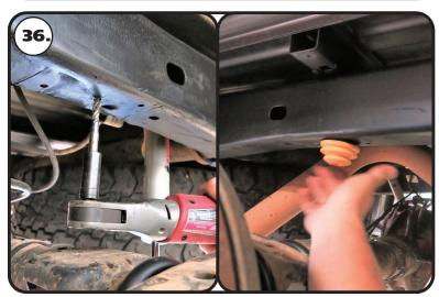
**36.** A hole will need to be drilled and tapped to 3/8"-16 to install the bump stop. This hole needs to located directly above the center of the axle. Mark the location and drill with a 5/16" drill bit. Tap the hole 3/8"-16. Thread the supplied bump stop into the hole until it is tight. Repeat on the other side.
