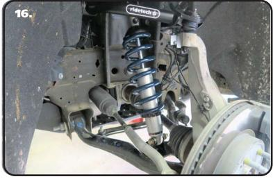
**16. Image 16** shows the CoilOver installed. Repeat steps 4-15 on the other side of the truck. Preload the springs of the CoilOver 1/2" to start. You may need to adjust the amount of preload in the spring, but this will be determined after the truck has been sat on the ground. Refer to **Page 9** for spring adjustment.
