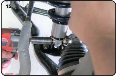
**15.** Install a 1/2" flat washer and 1/2"-13 nylok nut on the threads of the bolt that are sticking through the mount. Torque the upper and lower mounting hardware to 75 ftlbs.
