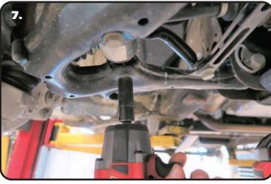
**7.** Remove the 2 lower shock/spring mounting bolts. The OEM shock/spring can now be removed from the truck.
