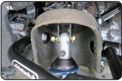
**13.** Install a 1/2" flat washer and 1/2"-13 nylok nut on the threads of the bolt that are sticking through the mount.
