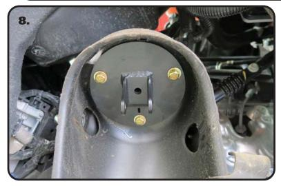
**8.** Install a 3/8" flat washer on each of (3) 3/8"-16 x 1 1/4" hex bolts. Align the mounting holes of the upper mount with the mounting holes in the frame. THE SLOT IN THE UPPER MOUNT, NEEDS TO BE TOWARD THE FRAME. The mounting bolts need to be installed with the threads pointing up. Insert a bolt/washer in each hole. Install a 3/8" flat washer and 3/8"-16 nylok nut on the threads of each bolt sticking through the frame. Torque the hardware to 45 ftlbs.
