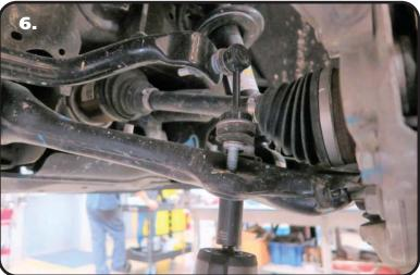
**6.** Remove the lower nut from the lower sway bar linkage. This will allow the suspension to be lowered easier for CoilOver removal and installation.
