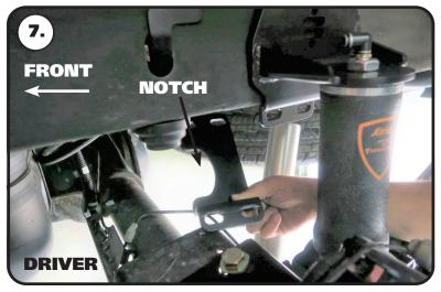
**7.** The inner frame plate is side specific. THE DRIVER SIDE HAS A NOTCH THAT WILL NEED TO BE POSITIONED TO THE FRONT OF THE TRUCK. The passenger side does NOT have a notch.
