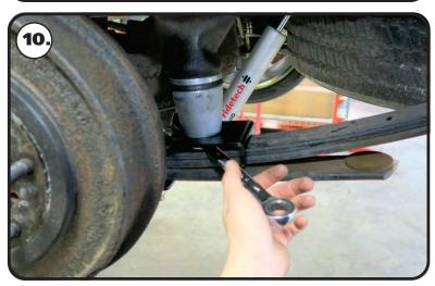
**10.** Tighten the lower 3/8" air spring bolt using a 9/16" wrench.
