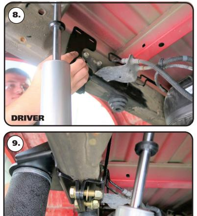
**8.** Hold the inner plate in position. It is bent to wrap under the frame rail. The (4) bolt holes will line up with the bolt holes of the upper air spring mount.
