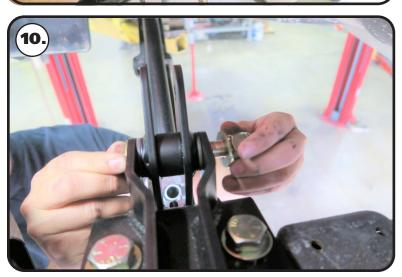
**10.** Install a 5/8" flat washer on a 5/8"-18 x 3 3/4" bolt. With the mounting holes aligned with the pivot inner sleeve, insert the bolt/ washer. Install a 5/8" flat washer & 5/8"-18 nylok nut on the bolt. Torque to 115 ft-lbs.
