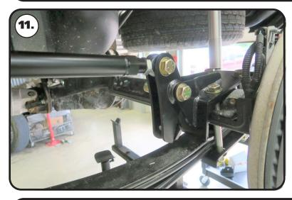
**11.** Insert the rear heim end into the ears of the axle pivot. Align the mounting holes with the through hole of the rod end. Install a 5/8" flat washer on a 5/8"-18 x 2 1/2" bolt. Insert the bolt/washer though the aligned holes. Install a 5/8" flat washer and 5/8"-18 nylok nut on the threads of the bolt. Torque to 115 ft-lbs. Repeat **Steps 3-11** for the other side.
