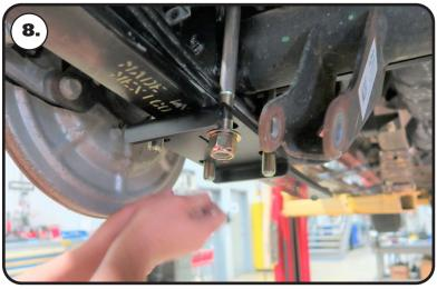
**8.** Instal a 5/8" flat washer on each of (4) 5/8"-18 x 7 1/2" hex bolt. Insert the bolt in through the axle mount. Slip the lower leaf spring bracket up onto the U-Bolts WITH THE OFFSET HOLE FORWARD. THE ARROW ON THE BRACKET SHOULD POINT TO THE FRONT OF THE TRUCK. Hold the Leaf Spring Bracket in place and install a 5/8" Flat Washer & 5/8"-18 Nylok Nut on the threads of the u-bolts. Snug the nuts down evenly and tighten them in a criss-cross fashion to 130 ftlbs
