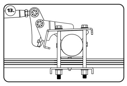
**13.** WITH THE TRUCK ON THE GROUND, THE SET LENGTH OF THE BARS NEED TO BE CHECKED. The bars need to be set so there is approximately 1/8" gap between the bumpstop and axle mount. Adjust the traction bar to get this gap set. After you check the gap, tighten the jam nuts on the traction bar.
