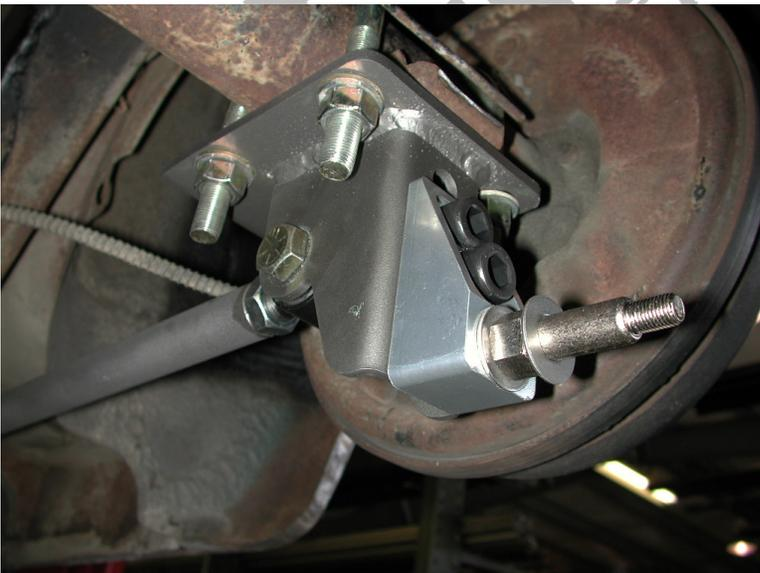
10. Secure the axle mount to the leaf spring pad using the supplied U-bolts. There is an aluminum bushing that will slide over the alignment pin.
