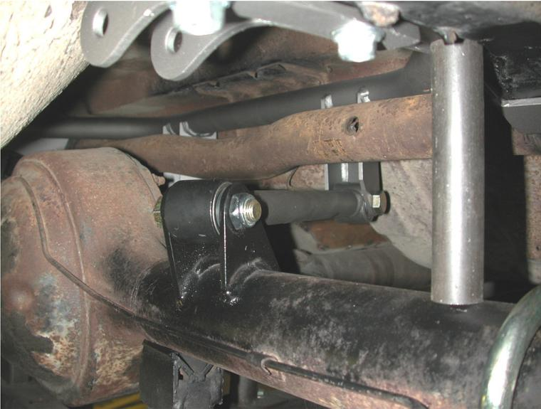
14. Bolt the axle tabs to the upper bar using a 5/8" x 2 3/4" bolt and nyloc as shown in the picture. The upper bar should measure 12" C-C.
