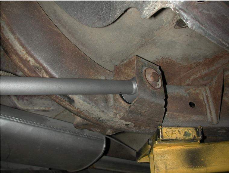
8. Bolt the large end of the lower bar (longer one) in the factory leaf spring mount using the factory bolts.
