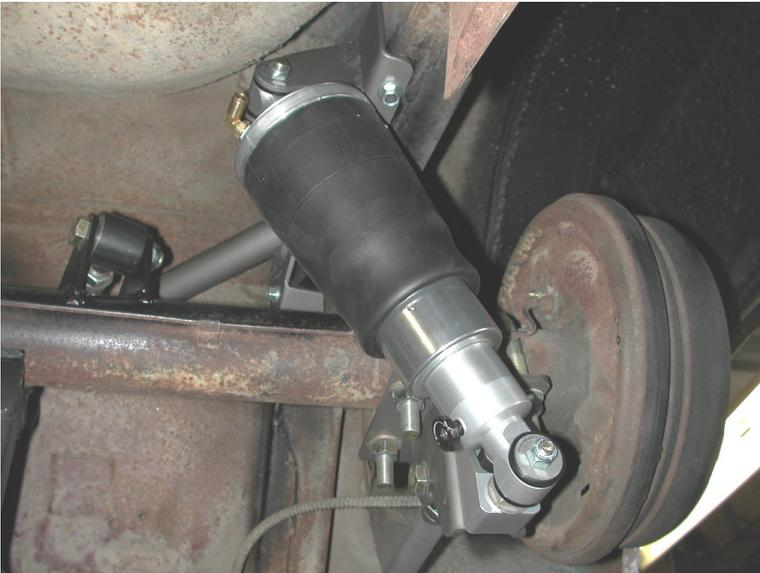
17. This must all be set at **ride height**, which will occur with 14.5" from c-c on the Shockwave mounts. As you can see in the above picture, we have tack welded a 5" long spacer between the axle and frame to maintain ride height, axle center, and pinion angle while welding in the tabs.
