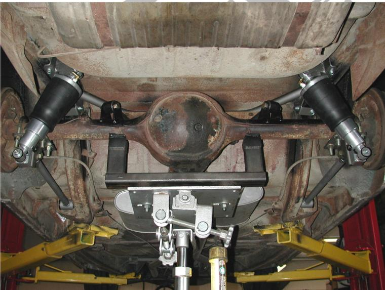
19. Apply thread sealant to the air fitting and screw it into the top of the Shockwave.
