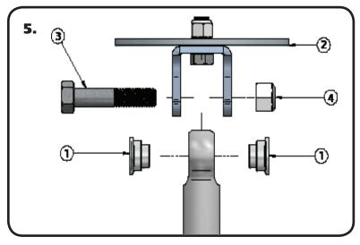
**5.** With the CoilOver assembled (**Refer to Page 3 for CoilOver assembly instructions**) insert the **NARROW** upper spacers(1) into the upper shock bearings. Install the **WIDE** spacers into the Lower Shock Bearing. With the spacers installed insert the CoilOver assembly into the upper shock mount(2). Align the holes in the bracket with the hole in the Shock spacers and insert the 1/2 x 2 1/2"" Bolt(3) and secure with the 1/2" Nylok Nut(4).
