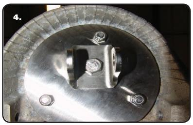
**4.** Install the upper mount into the crossmember using (3) 5/16" x 1 1/2" Hex Bolts, (3) 5/16" SAE Flatwashers, & (3) 5/16" Nylok Nuts. Position the Straight edge of the Mount facing the Engine Compartment. Tighten the mounting hardware.
