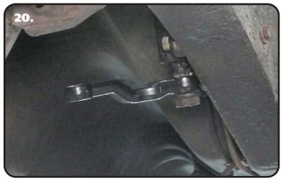
**20.** The TruTurn kit includes a new pitman arm. A pitman arm puller is necessary to replace the pitman arm. Remove the OEM pitman arm using a pitman arm puller. If you do not have one, they can usually be rented from your local auto parts store. Install the new pitman arm using **Image 20** as a reference. The large diameter of the centerlink pin taper should be down toward the ground. Torque the nut 85-110 ftlbs.-+
