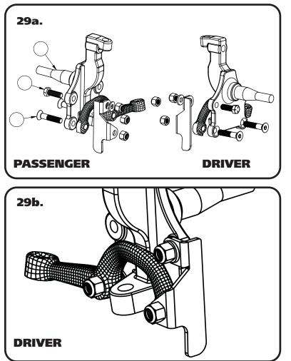
**29a.** Install the steering arms and steering stops onto the spindle using **Images 29a & 29b** as a reference. The steering arms angle toward the centerlink, and the tie rod mounting holes are to the rear of the car. The steering stops are marked D and P.
