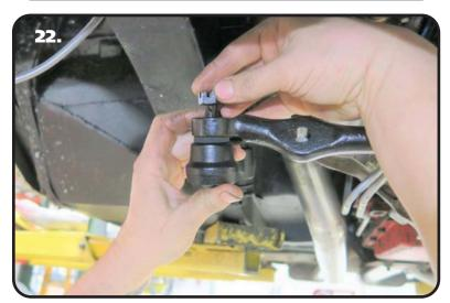
**22.** The other end of the centerlink will sit down on the stud of the idler arm. Install the end of the centerlink on the stud and torque the castle nut to 25-30 ftlbs. Tighten the nut to align the cotter pin. Install the cotter pin and bend the ends.
