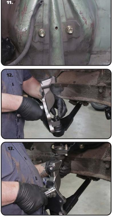
**11.** Install a 1/2" flat washer, 1/2" split lock washer, and 1/2"-13 nut on the threads of the 2 bolts sticking through into the engine compartment. Torque to 75 ftlbs.
