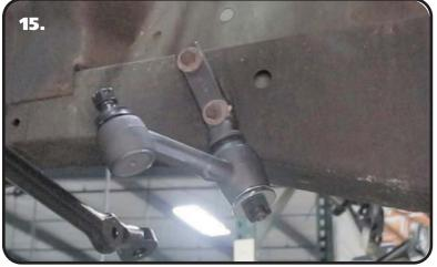
**14.** Remove the idler arm that is currently installed on the car. Your current idler arm may have 3 mounting holes, but there is a 2 hole bolt pattern under it. The idler arm supplied with the kit will use the 2 mounting holes circled in **Image 14**.
