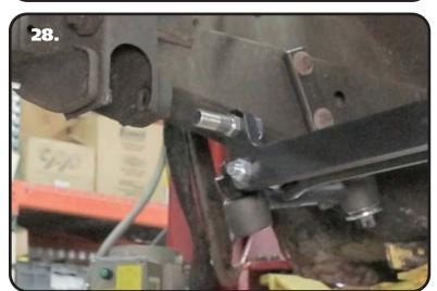
**26.** Install the 1/2"-20 mechanical locking nuts and torque to 50 ftlbs.
