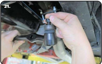
**21.** Attach the new centerlink in the pitman arm. The centerlink only has a tapered pin on one end, it goes into the pitman arm. Torque the nut of the centerlink pin to 35-47 ftlbs and tighten to align the cotter pin hole. Install the cotter pin and bend the ends.
