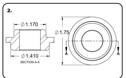
**2.** This kit includes a t-bushing for the strut rod bushing factory hole. The factory hole can be 2 different diameters depending on the year of the car. The size of your frame hole will determine which direction the t-bushing is installed.
