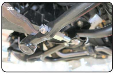
**23.** The studs with the long hex on them will get installed into the factory centerlink with the taper going into the centerlink, a 7/16" castle nut is used to attach it to the centerlink. The straight shank will point to the front of the car.
