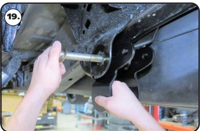
**19.** Install a M18 flat washer on a M18-2.5 x 130mm bolt. Insert the bolt into the OEM leaf spring hole. Install a M18 flat washer & M18-2.5 nylok nut on the threads of the bolt. Do not tighten at this time.
