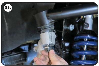
**31.** Insert the ball joint stud into the spindle. Install the flat washer supplied with the ball joint nut. Next, install the ball joint nut and torque to 50 ft-lbs. Tighten the nut until a slot in the nut aligns with the hole in the ball joint pin. NEVER LOOSEN THE NUT TO ALIGN THE HOLE!
