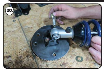
**20.** Install the 1/2" I.D. bearing spacers into the bearing in the shock eyelet. These spacers have a through hole that is 1/2" diameter. The small diameter of the spacers will insert into the shock bearing.
