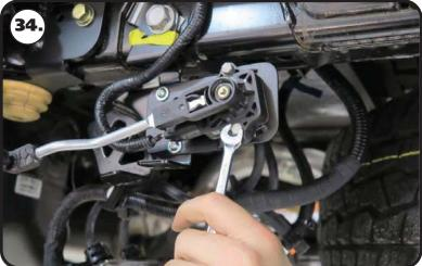
**34.** Reinstall the headlight sensor on the new bracket using the OEM hardware. The new bracket is slotted to allow for adjustment to set the headlights to your new ride height.
