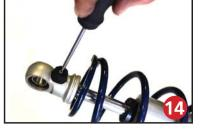
Before the upper spring mount can be installed screw the adjuster knob on the upper eye mount to the firmest setting (clockwise) as seen in figure 8. Then remove the Knob by holding it while removing the center screw.
