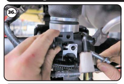
**36.** The lower relocation bracket will get positioned under the brake line mount. The tab of the brake line mount needs to be engaged in the bracket and leaf spring pad. Reinstall the OEM hardware if you're not running the helper air spring kit. If you are using the helper air spring kit, use the supplied M8-1.25 x 30mm bolt and M8 flat washer. Torque to 169 in-lbs.
