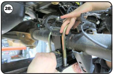
**28.** Slip the u-bolts over the axle tube with the threads pointing down.
