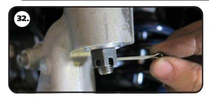
**32.** Install the supplied cotter pin. Bend the tabs of the cotter pin.
