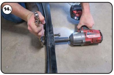
**14.** Remove the locating pins from the leaf spring pack. Reinstall the locating pins from the TOP side. Reinstall the nuts on the BOTTOM side and tighten. Torque the nuts to 35 ftlbs Repeat on the second spring.
