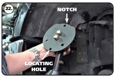
**22.** The upper mount has 4 holes in the perimeter of the flange. The flange is also notched out on one side. The upper mount needs to be installed in the truck with the notch to the frame.
