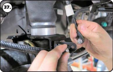
**37.** Reattach the headlight sensor linkage to the new bracket.
