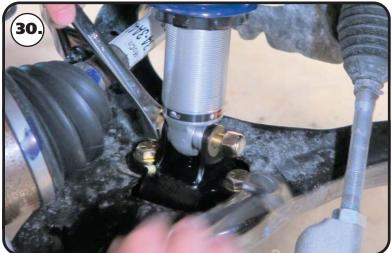
**30.** Install a 1/2" flat washer and 1/2"-13 nylok nut on the threads of the bolt that are sticking through the mount.
