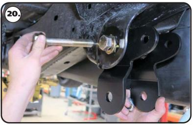
**20.** Make sure the holes in the front tab line up with the front hole of the OEM leaf spring mount. Install a 3/4" flat washer on a 3/4"-16 x 5" bolt. Insert the bolt/washer through the front hole of the leaf spring mount. Install a 3/4" flat washer & 3/4"-16 thin nylok nut on the threads of the bolt. Torque the hardware to 75 ftlbs.
