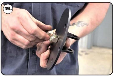
**19.** Install a 1/2" SAE flat washer & 1/2"-13 nylok nut on the threads of each bolt that is sticking through the mount. Torque to 75 ftlbs.
