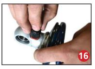
Install upper spring mount retainer clip (803-00-199) into the groove on the upper eyelet as seen in figure 10. Then, reinstall adjuster to complete assembly.
