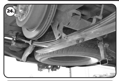
**24.** Raise the axle high enough to get the flip bracket positioned on the leaf spring.
