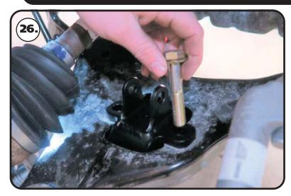
**26.** Install a 1/2" flat washer on each of (2) 1/2"13 x 3" hex bolts. Insert a bolt/washer in each mounting hole.
