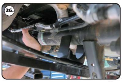
**26.** Position the flip bracket on the locating pins. Again, the locating pin holes go to the front of the truck.
