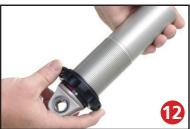
First, using the supplied lower adjuster nut (803-00-199) thread the nut onto the shock from the bottom side as seen in figure 6. Remove the plastic pellet that is in the split of the adjuster nut.
