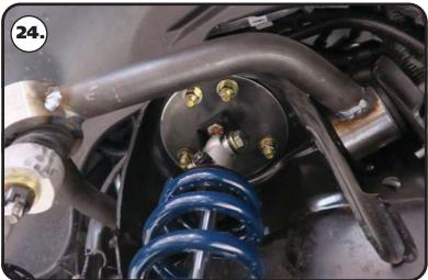
**24.** Install a 7/16" flat washer on each of (4) 7/16"-14 x 1 1/4" hex bolts. Install the bolt/ washer in the frame/mount from the top side with the threads pointing down. Install a 7/16" flat washer and 7/16"-14 nylok nut on the threads of each bolt sticking through the frame. Torque the hardware to 50 ftlbs. Repeat steps 17-24 on the remaining side.
