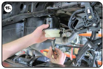
**15.** The OEM bump stop mount will need to be removed.
