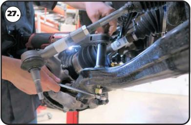
**27.** Install a 1/2" flat washer and 1/2"-13 nylok nut on the threads of each bolt sticking through the control arm. Torque the hardware to 75 ftlbs.
