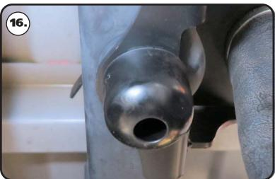
**16.** Install a M10 flat washer on a M10-1.5 x 30 mm socket head cap screw. Insert the washer/bolt in the center hole of the bumpstop. Use a hex key (allen) wrench to attach the bumpstop in the OEM location. Repeat on the other side and torque to 35 in-lbs.
