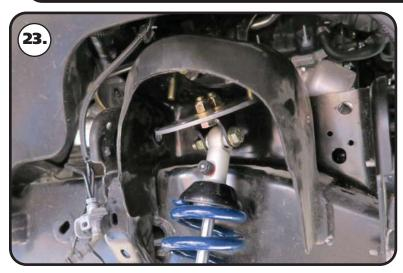
**23.** Position the mount/coilover in the truck. It will be placed in the OEM location. Line up the locating hole and 3 mounting holes.
