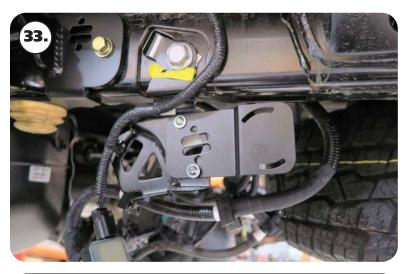
**33.** Align the relocation bracket holes with the mounting holes of the OEM bracket. Attach the new bracket using the supplied 10-24 x 3/4" bolts/ washer and nylok nuts. Tighten to 22 in-lbs.
