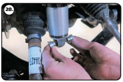
**28.** Install the 1/2" I.D. bearing spacers into bearing in the shock body. These spacers have a through hole that is 1/2" diameter. The small diameter of the spacers will insert into the shock bearing.
