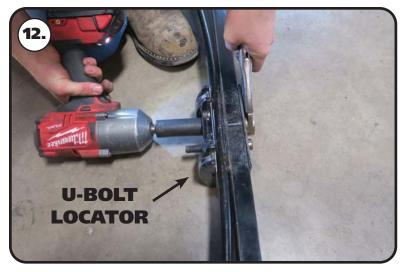
**12.** The leaf spring locating pins need to be flipped over. Currently, the nuts for the pins are on the top side of the leaf spring pack. The nuts will need to be on the bottom side for proper location of the flip bracket. The u-bolt locating plate will need to be removed and discarded. The pins can be held with a pair of vise grips to loosen and remove the nuts.
