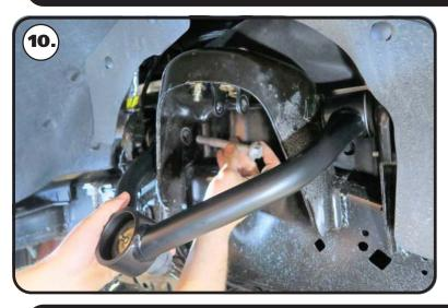
**7.** Install the Ridetech upper control arms using the OEM hardware. Again, the drivers side control arm has a headlight sensor tab on it. If installing controls arms on a 2021 F150, reattach the headlight sensor linkage to the tab of the control arm. The control arm mounting bolts will need to be tightened after the truck is sitting on the ground.
