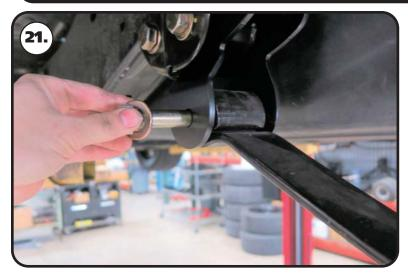
**21.** Insert the front of the leaf spring in the new bracket. Install a M18 flat washer on a M18-2.5 x 130mm bolt. With the mounting holes aligned with the inner sleeve of the leaf spring, insert the bolt/washer. Install a M18 flat washer and M18-2.5 nylok nut on the threads of the bolt. Re peat on the second side. Do not tighten this hardware until the truck is sitting on the ground
