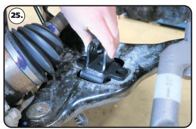
**25.** The lower shock mount bolts to the lower control arm in the same location as the OEM shock. Sit the mount on the lower control arm, aligning the mounting holes with the shock mounting holes
