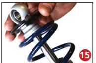
Once the knob is removed slide a Delrin washer over the eyelet. Next, slide the upper spring mount (803-00-199) over eyelet as seen in figure 9.
