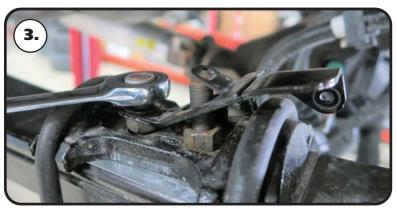
**3. 2021 ONLY!** Disconnect the headlight sensor linkage from the Drivers side leaf spring mount. Remove the linkage bracket from the axle. There isn't a sensor on the Passenger side of the truck.
