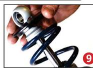
Once the knob is removed slide a Delrin washer over the eyelet. Next, slide the upper spring mount (803-00-199) over eyelet as seen in figure 9.
