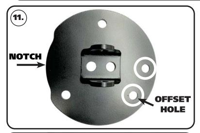
**11.** Line up the 2 mounting holes in the upper mounting flange with the 2 holes of the mounting bracket. The location of the offset hole is critical. Make sure it is located the same as **Image 11**. The front hole is a locating hole.
