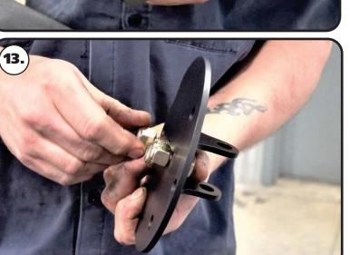
**13.** Install a 1/2" SAE flat washer & 1/2"-13 nylok nut on the threads of each bolt that is sticking through the mount. Torque to 75 ftlbs.
