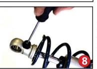
Before the upper spring mount can be installed screw the adjuster knob on the upper eye mount to the firmest setting (clockwise) as seen in figure 8. Then remove the Knob by holding it while removing the center screw.
