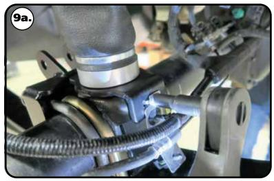
**9a. & 9b.** The lower mount gets attached with the M8-1.25 x 30mm & M8 flat washer supplied with the kit. **9a** is 2015-2020 F150, it has no headlight sensor. **9b** is 2021 F150 WITH a headlight sensor on the driver side. Align the rear tab of the lowering mount with the mounting hole in the leaf spring mount. Install the M8 flat washer on the M8-1.25 x 30 mm bolt and thread it into the OEM mounting hole. Torque to 169 in-lbs.
