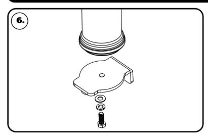
**6.** Attach the lower air spring mount to the bottom of the air spring using a 3/8"-16 x 1" bolt, 3/8" split lock washer, & 3/8" SAE flat washer. Torque to 23 ft-lbs. Repeat for the 2nd air spring & mount.
