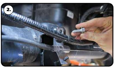
**2.** Remove the brake line bracket bolt from the rear of the leaf spring pads.
