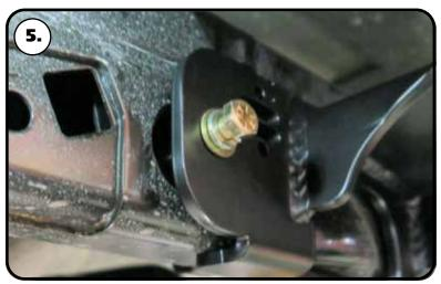
5. Install a 3/8" split lock washer & 3/8" SAE flat washer on each of (2) 3/8"-16 x 1 3/4" hex bolts. Apply Red Loctite to the threads of each bolt. Insert the bolts into each mounting hole in the side of the upper air spring mount. Thread each bolt into a nut plate. Torque the bolts to 30 ft-lbs.
