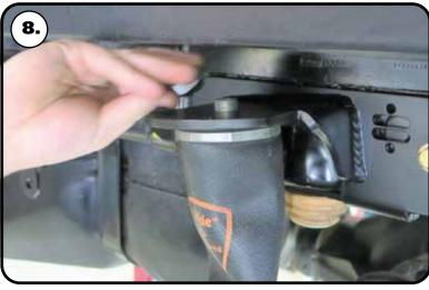
**8.** Thread the 3/4"-16 jam nut on the upper stud of the air spring, but do not tighten until at this time.
