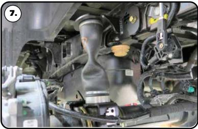
7. Insert the air spring into position with the upper mounting stud through the 3/4" hole in the upper mount. The long tab of the lower mount will go against the rear of the leaf spring mount of the axle.
