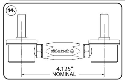
**14.** Set the Linkage to 4 1/8" center to center with the threaded studs pointed the same direction. Snug the jam nuts against the center adapter. Use **Diagram 14** as a reference.
