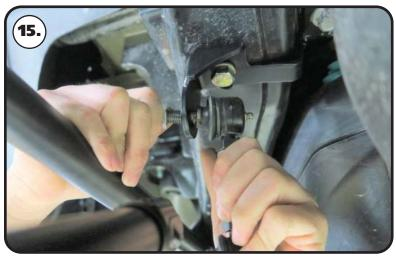
**15.** Attach the linkage to the frame bracket with the threads of the end link pointing outward. Use the hardware on the linkage to attach it. Torque the nut to 37 ft-lbs. Repeat on the other side.
