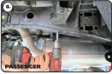
**8.** Drill the passenger side shock crossmember using a 1/2" drill bit. We user the back edge of the frame slot as a guide. Drill the whole straight up from the rear of the frame slot.
