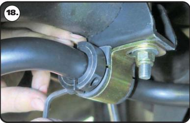
**18.** Install the locking rings on the inside of each bushing assembly. Use a hex key to take the locking ring apart. Reassemble it on the bar positioned next to the inside of the bushing assembly. Push the locking ring up against the bushing assembly and tighten.
