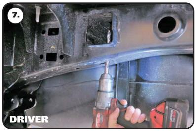
**7.** The gas tank/shock crossmember will need to be drilled to attach the frame mount. We use the rear of the frame slot as a guide. Drill the crossmember straight above the frame slot using a 1/2" drill bit.
