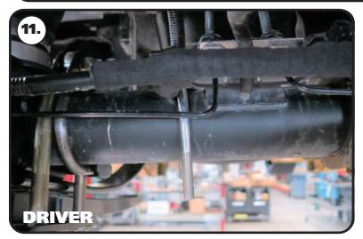
**11.** Install a 7/16" u-bolt on the driver side axle tube just to the outside of the brake line mount.
