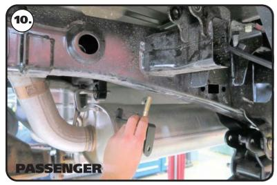
**10.** Repeat the above steps on the passenger side using the LONG nut plate to hold the frame mount.
