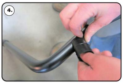
**4.** Open the delrin liner at the split and slip it over the sway bar. Position it in the center of the straight area that it will ride in. Do this on both ends of the sway bar.
