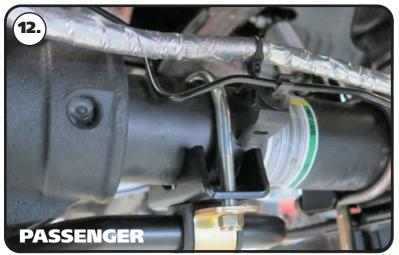
**12.** Install a 7/16" u-bolt on the passenger side axle tube just to the inside of the brake line bracket.
