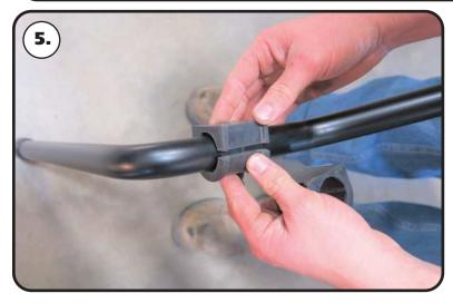
**5.** Open the sway bar bushing at the split and slip it **OVER** the delrin liner. Do this on both delrin liners.
