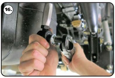
**16.** Install a T-Bushing on each of the bottom 90 degree end links. The t-bushings are installed with the large diameter against the shoulder of the end link. Insert the 90 degree end link/t-bushing into the swaybar end with the threads pointing outward.
