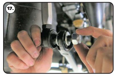
**17.** Install a 2nd t-bushing with the small diameter into the swaybar. Install the nut and torque to 37 ft-lbs. Do this for both sides.
