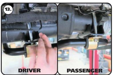
**13.** Hold the sway bar in position on the truck with the center bend toward the ground. Install a 7/16" Flat Washer & 7/16"-20 Nylok Nut on the threads of the u-bolts. The axle mounts should be positioned parallel with the leaf springs. Snug the hardware down and verify the axle mounts are parallel with the leaf springs. Torque the u-bolt hardware to 35 ft-lbs.
