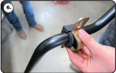
**6.** Install the bushing straps over the sway bar bushings.
