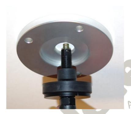
3. Bolt the aluminum upper plate to the car in place of the factory rubber mount using the 3/8" x 1 1/4" bolts, flat washer and Nylok nuts.
